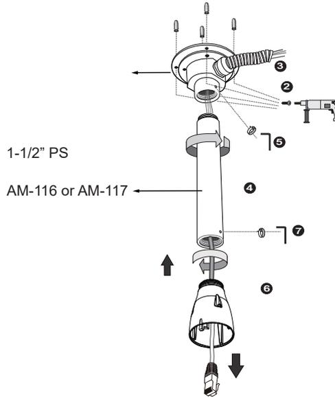
4. Connect the Ethernet cable to the camera. When inserting the camera, align the camera's embedded **microphone** with the triangle indent on the pendant adaptor.
