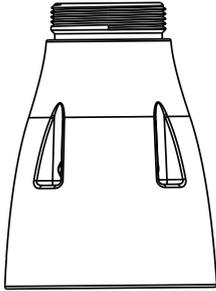
3. Remove the retention springs on the sides of the camera.
